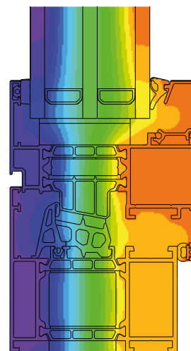
Distribution of isotherms in MB-79N SI window
